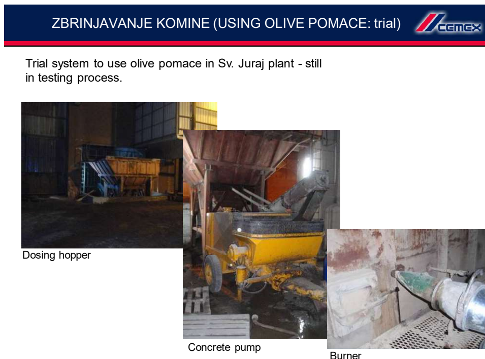
Slika 15. Proces zbrinjavanja komine izvor: Plan for sustainable CEMEX in Croatia, June 2010, archive
